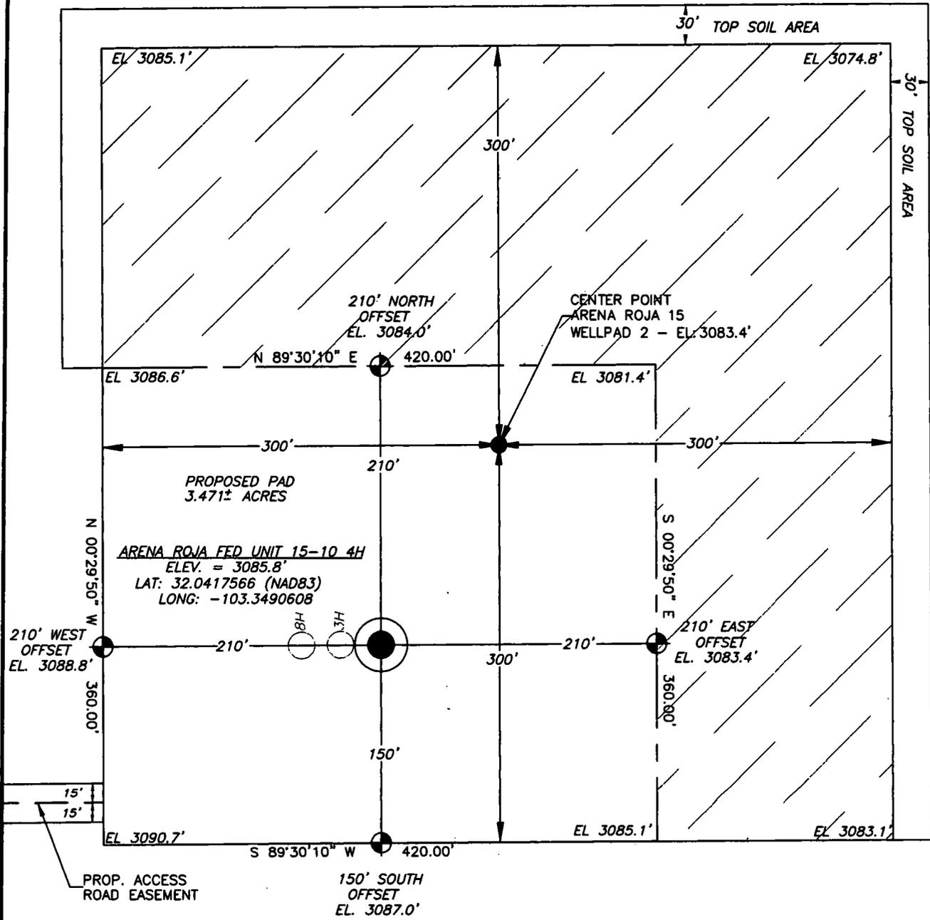
Note: All bearings recited herein are based on the New Mexico State Plane Coordinate System, NAD 83, New Mexico East Zone 3001, US Survey Feet, all distances are grid.
