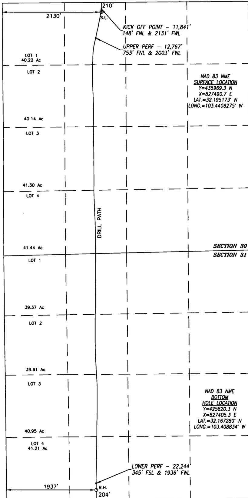
SURFACE INFO AND BOREPATH SHOWN HEREBON IS BASED ON DIRECTIONAL SURVEY REPORT PROVIDED BY COG OPERATING, LLC FOR THE FASCINATOR FEDERAL COM #601H SUPPLIED TO HARCROW SURVEYING, LLC ON OCTOBER 4, 2019
