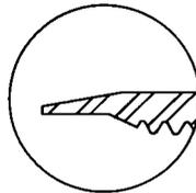
Casing Special Clearance Coupling 10° Bevel
