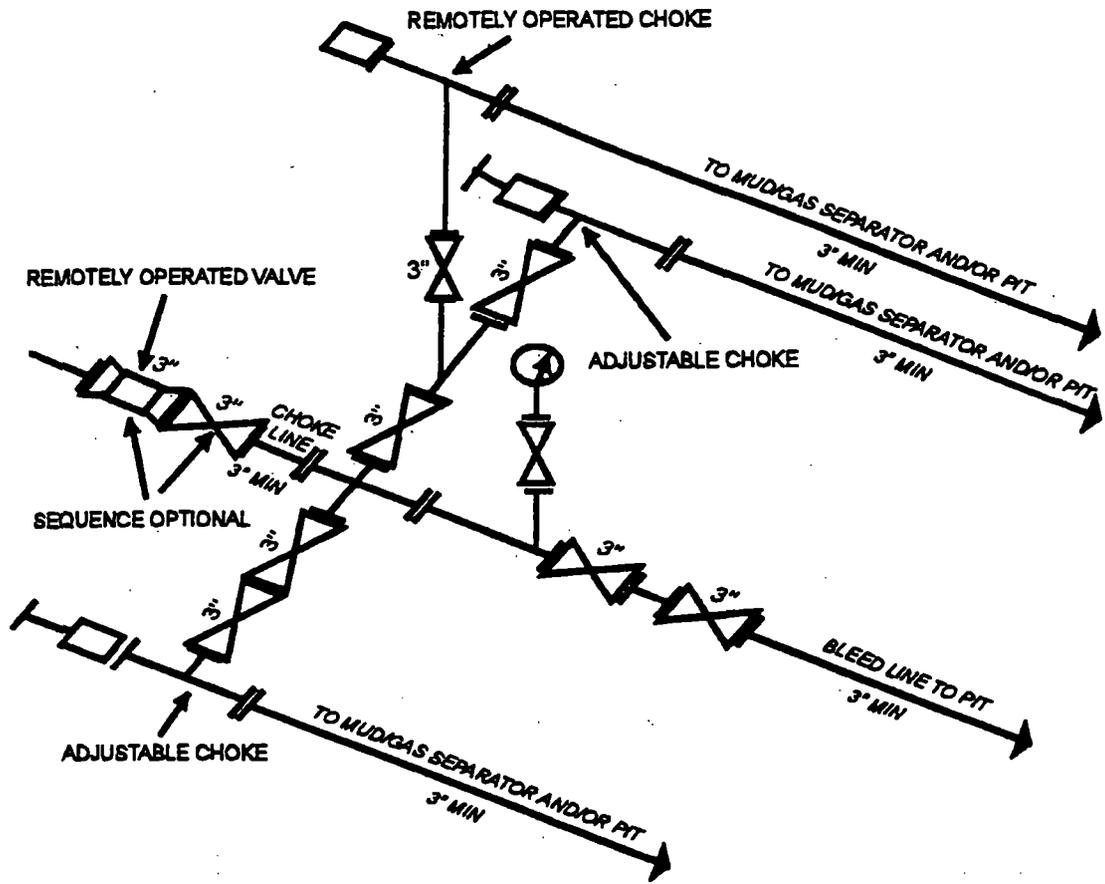
**10M AND 15M CHOKE MANIFOLD EQUIPMENT - CONFIGURATION OF CHOKES MAY VARY**
