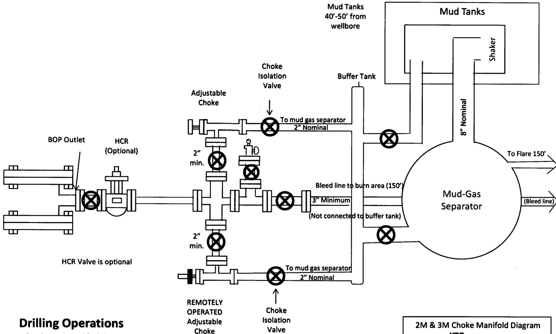
2M & 3M Choke Manifold Diagram
