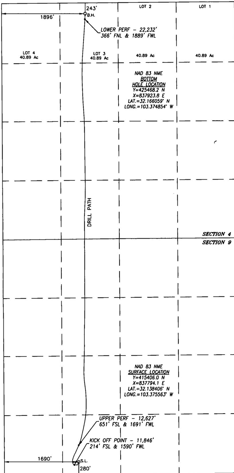
SURFACE INFO AND BOREPATH SHOWN HEREON IS BASED ON DIRECTIONAL SURVEY REPORT PROVIDED BY COG OPERATING, LLC FOR THE FEZ FEDERAL COM #602H SUPPLIED TO HARCROW SURVEYING, LLC ON NOVEMBER 15, 2019
