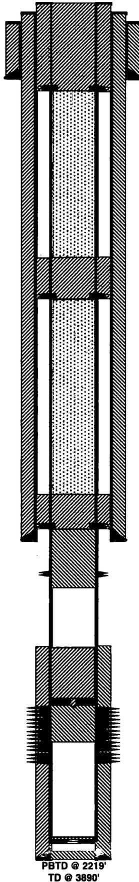
3. PUH & perf @ 250' & sqz 75 sx Class "C" cmt from 250' to surf. Attempt to CIRC 6 5/8" to surf. (Surf Shoe & Water Board)
