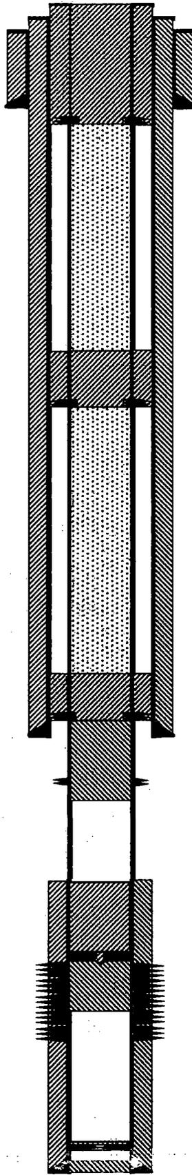
3. PUH & perf @ 250' & sqz 75 sx Class "C" cmt from 250' to surf. Attemp to CIRC 6 5/8" to surf. (Surf Shoe & Water Board)
