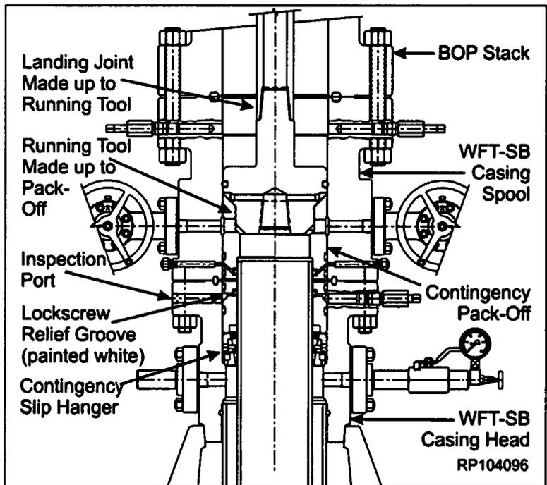
11. Verify, through inspection port that the pack-off bushing has landed properly after:
