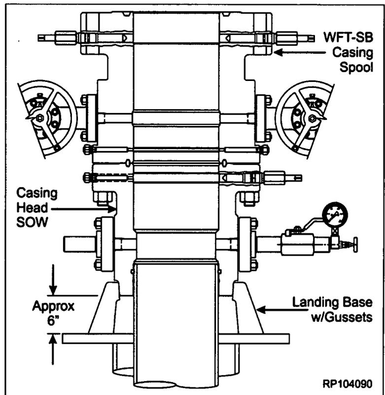
10. Determine the correct elevation for the wellhead assembly. Measure depth of the surface casing socket in SOW with O-ring bottom prep.
