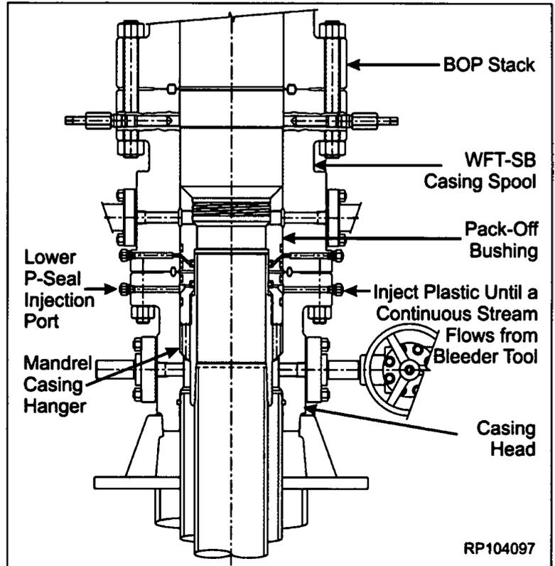
5. Lower the test plug through the BOP stack into the WFT-SB spool assembly until it lands on top of the pack-off bushing.
