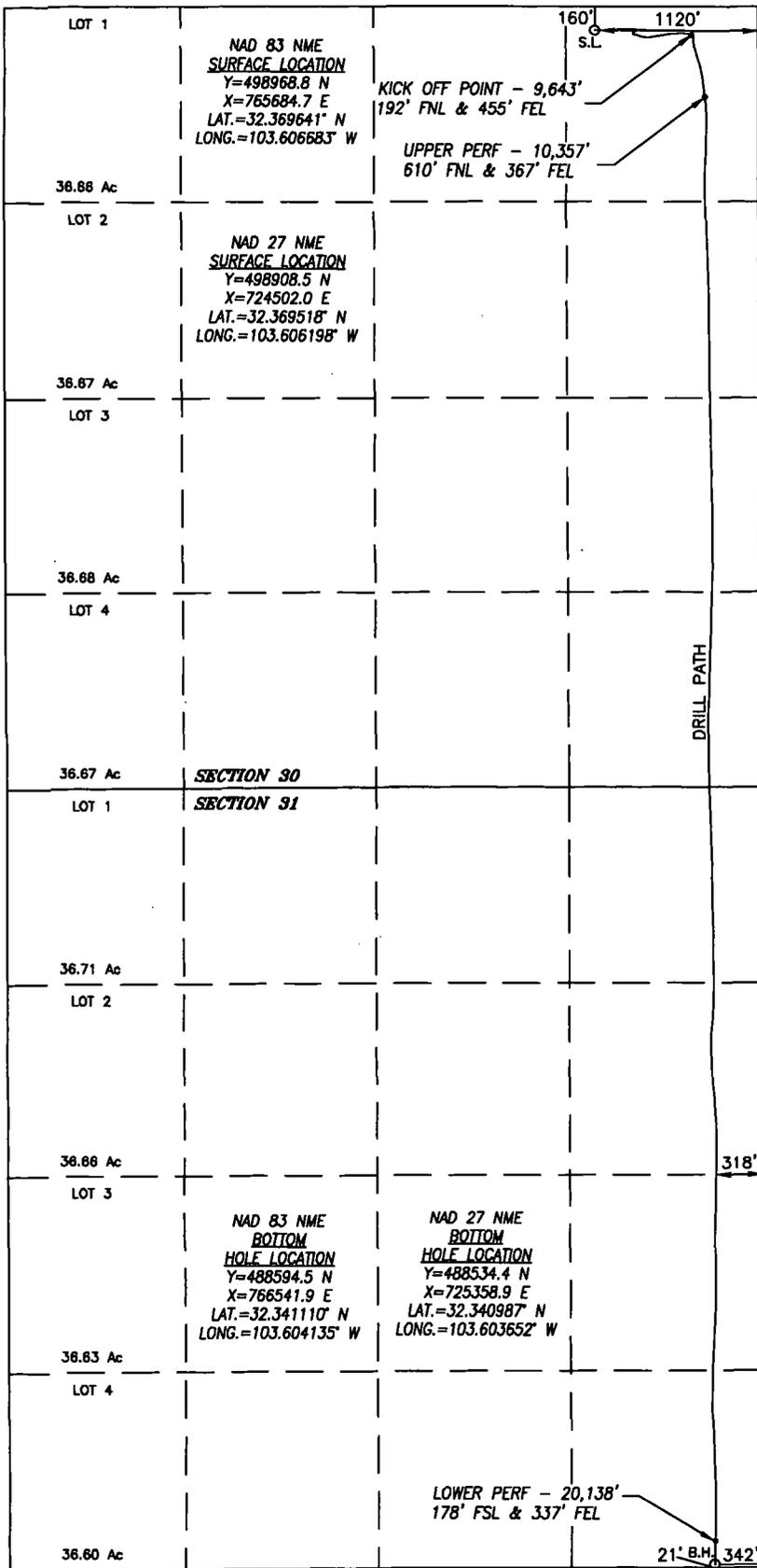
SURFACE INFO AND BOREPATH SHOWN HEREON IS BASED ON DIRECTIONAL SURVEY REPORT PROVIDED BY OXY USA FOR THE AVOGATO 30\_31 STATE COM 4H SUPPLIED TO HARCROW SURVEYING, LLC ON DECEMBER 20, 2019
