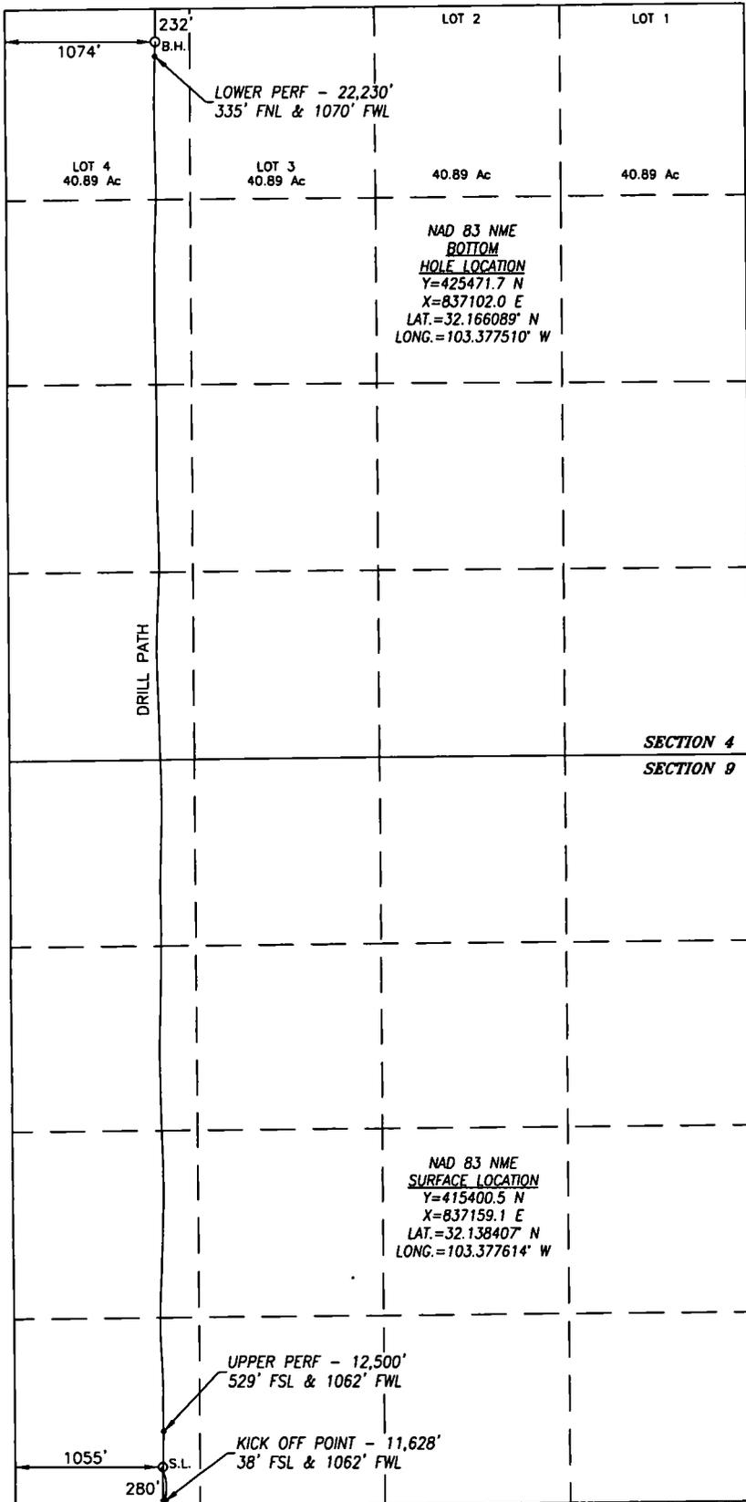
SURFACE INFO AND BOREPATH SHOWN HEREON IS BASED ON DIRECTIONAL SURVEY REPORT PROVIDED BY COG OPERATING, LLC FOR THE FEZ FEDERAL COM #603H SUPPLIED TO HARCROW SURVEYING, LLC ON NOVEMBER 18, 2019
