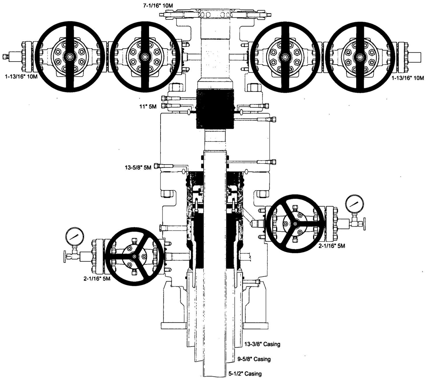
A multibowl wellhead may be used. The BOP will be tested per Onshore Order #2 after installation on the surface casing which will cover testing requirements for a maximum of 30 days. If any seal subject to test pressure is broken the system must be tested.
