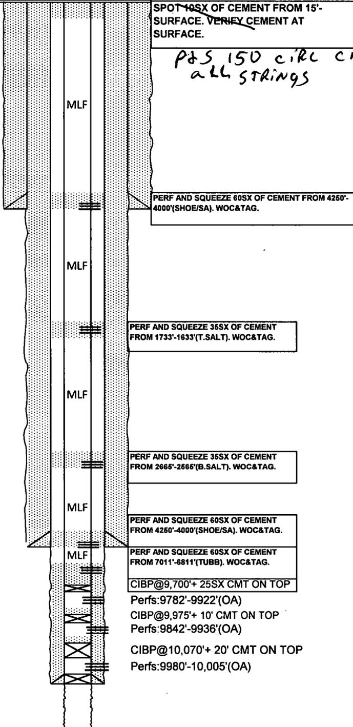
SPOT 10SX OF CEMENT FROM 15'-SURFACE. VERIFY CEMENT AT SURFACE.
