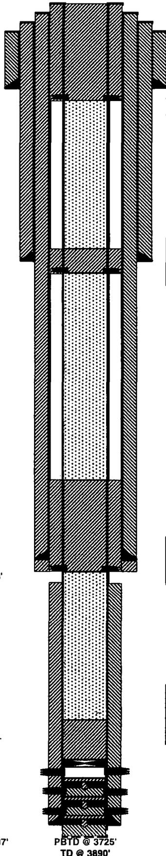
4. PUH & perf @ 318' & sqz/CIRC 70 sx Class "C" cmt from 318' to surf. Attempt to CIRC 7 5/8" to surf. (Surf Shoe & Water Board)
