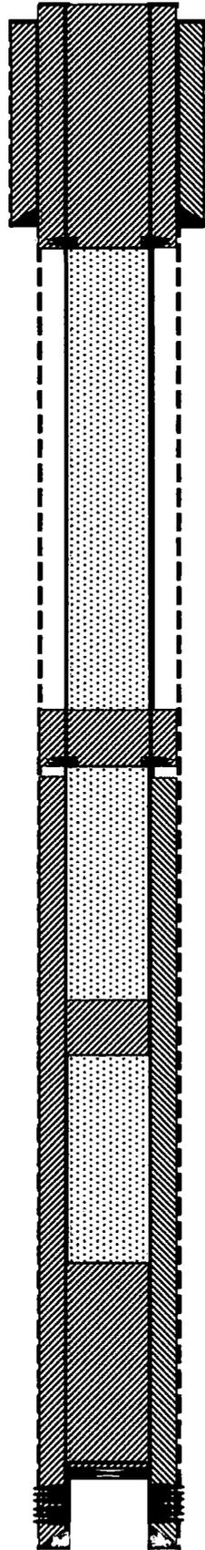
4. PUH & perf @ 445' & sqz 160 sx Class "C" cmt from 445' to surf. Attempt to CIRC 5 1/2" to surf. (Surf Shoe, Water Board, & Surf Plug)
