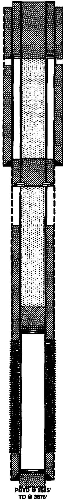
3. PUH & perf @ 300' & sqz/CIRC 220 sx Class "C" cmt from 300' to surf. Attempt to CIRC 7 5/8" & 10 3/4" to surf. (Water Board & Surf Plug)
