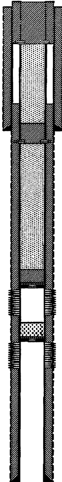
3. PUH & perf @ 250' & sqz 70 sx Class 'C' cmt from 250' to surf. Attempt to CIRC 5 1/2" to surf. (Water Board & Surf Plug)
