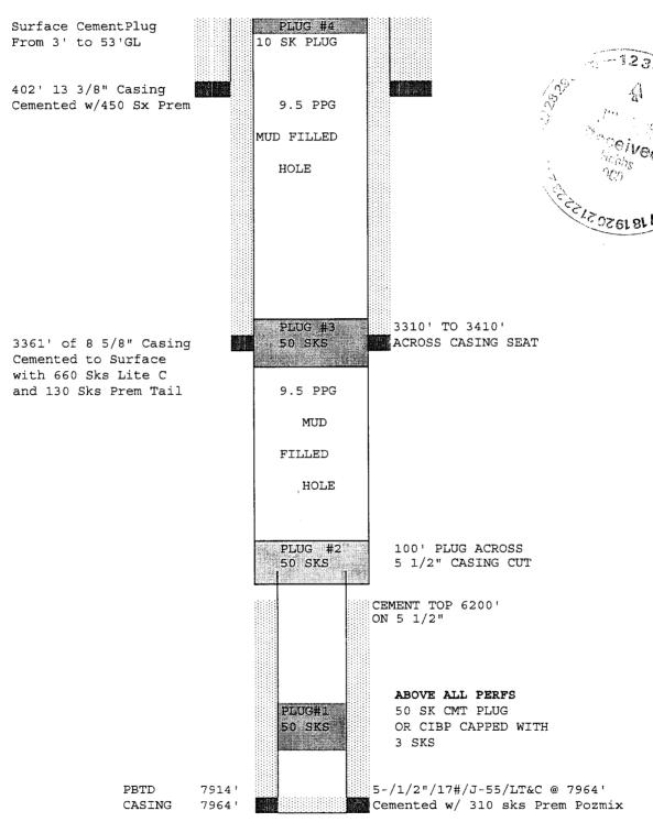
PROPOSED WELL BORE SCHEMATIC AFTER PLUGGING
