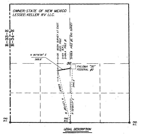
A STRIP OF LAND JO.O FEET WIDE, LOCATED IN SECTION 30, TOWNSHIP23 SOUTH, RANGE 34 EAST, N.M.P.M., LEA COUNTY, NEW MEXICO AND BEING 15.0 FEET LEFT AND RIGHT OF THE FOLLOWING DESCRIBED CENTERLINE SURVEY.
