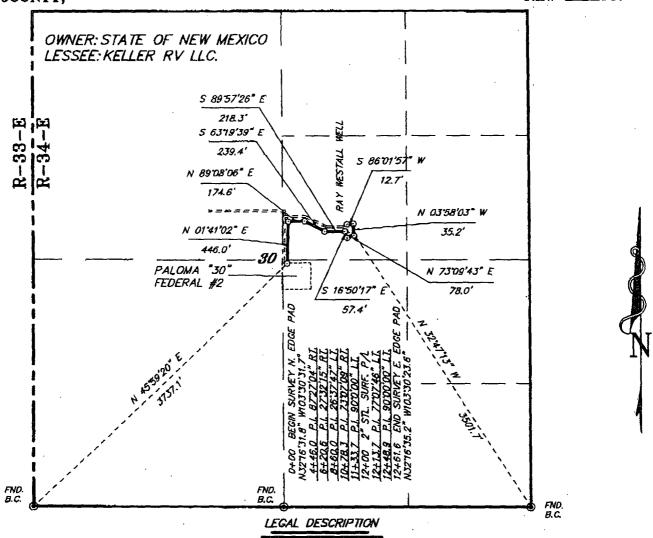
A STRIP OF LAND 30.0 FEET WIDE, LOCATED IN SECTION 30, TOWNSHIP 23 SOUTH, RANGE 34 EAST, N.M.P.M., LEA COUNTY, NEW MEXICO AND BEING 15.0 FEET LEFT AND RIGHT OF THE FOLLOWING DESCRIBED CENTERLINE SURVEY.
