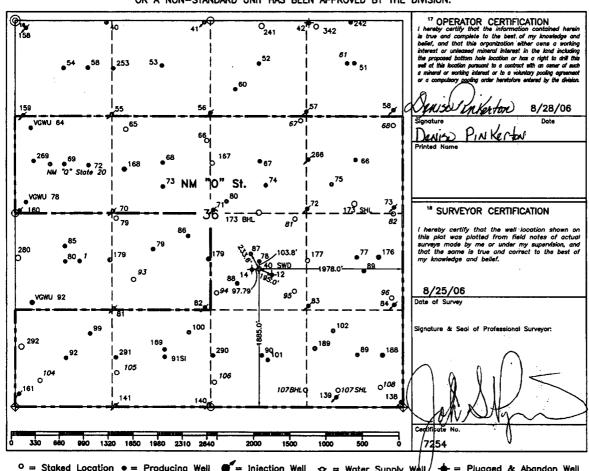
° = Staked Location • = Producing Well ✓ = Injection Well ✓ = Water Supply Well + = Plugged & Abandon Well O = Found Section Corner, 2 or 3" Iron Pipe & GLO B.C. o = Found /4 Section Corner, 1" Iron Pipe & GLO B.C.
