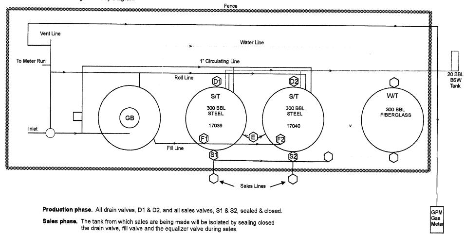
**Draining phase.** The tank being drained will be isolated by sealing closed the sales valve, fill valve, equalizer valve and the drain valves on the other tanks.
