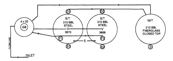
Production phase. All drain valves, D1 & D2, and all sales valves, S1 & S2, sealed & closed.
