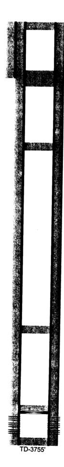
12-1/4" hole @ 498' 8-5/8" csg @ 498' w/350sx-TOC-Surf-Circ
