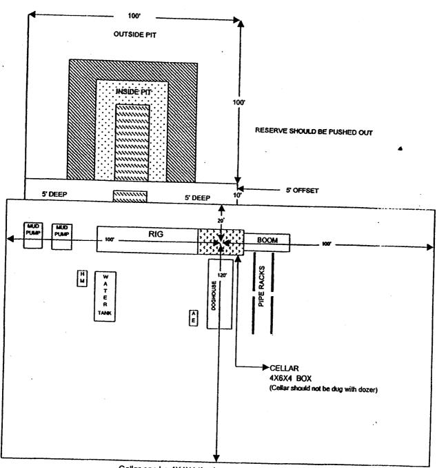
Cellar can be 4X4X4 if using a screw-on wellhead Working Pits dug 5' below ground level
