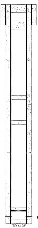
12-1/4" hole @ 325' 8-5/8" csg @ 325' w/275sx-TOC-Surf-Circ
