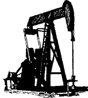
Emsco 114-C 54 in the 54" stroke running 6 spm
