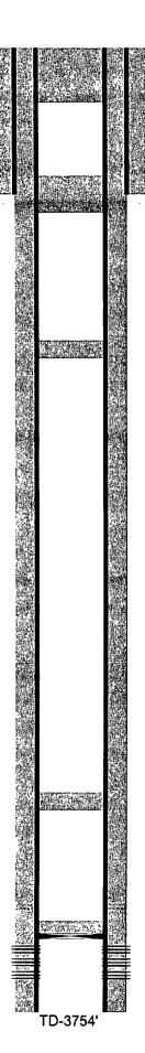
12-1/4" hole @ 530' 8-5/8" csg @ 530' w/275sx-TOC-Surf-Circ
