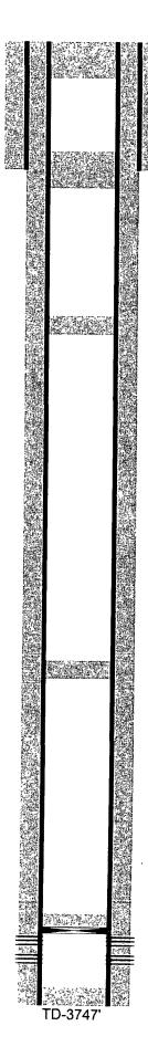
12-1/4" hole @ 507' 8-5/8" csg @ 507' w/400sx-TOC-Surf-Circ
