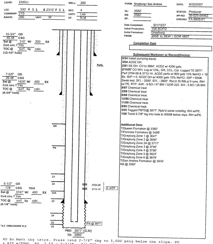
6 RIH w/BPML, PS, 2.5" x 2-3/4" x 24' THB pmp w/3' plngr (SN# EMSU1010), 7 jts 2-7/8", 6.5#, J-55, EUE, 8rd tbg, 5-1/2" TAC & 112 jts 2-7/8", 6.5#, J-55, EUE, 8rd tbg. Set TAC w/18 pts tens. NU WH. RIH w/1" on/off tool, 39 - 1" D-90 rods, 99 - 3/4" D-90 rods, 11 - 1" D-90 rods, 3 - 1" D-90 pony rods (6', 4' & 8') & 1-1/2" x 26' SM PR. Latched onto pmp. SWO & HWC. RU Key pmp trk. Loaded tbg w/15 BW. Press tbg to 500 psig in 1 stroke, shop).
