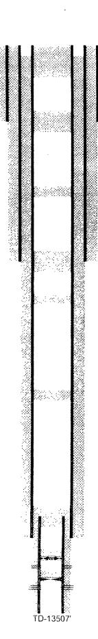
17-1/2" hole @ 1735' 13-3/8" csg @ 1735' w/1400sx-TOC-Surf-Circ
