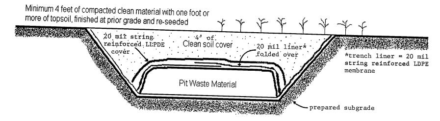
The length and width and depth of the on-site trench will be determined after calculating the volume of waste material compared to the depth to groundwater.
