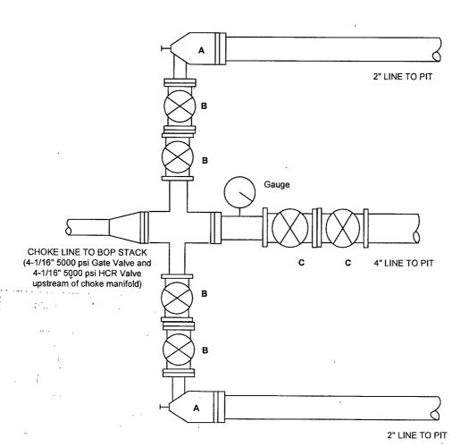
Choke Controls - At Least One Choke Also Remotely Controlled From Rig Floor
