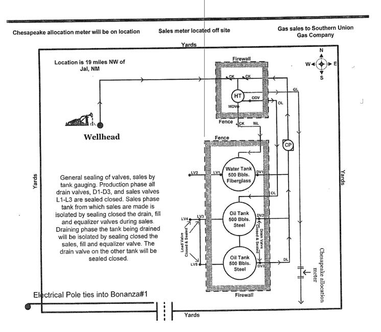
\*\* We will lay a 2" Poly gas line 220 'E to tie into Papagayo Federal #1 Gas line that will connect to Southern Union Gas Company sales meter \*\*
