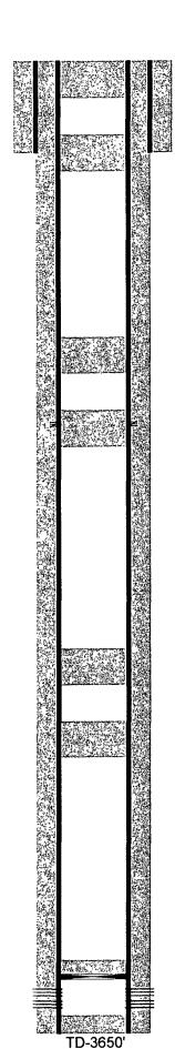
11" hole @ 351' 8-5/8" csg @ 351' w/ 150sx-TOC-Surf-Circ
