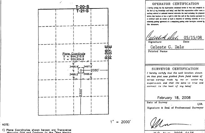
Plane Coordinates shown hereon are Transverse Mercator Grid and Conform to the "New Mexico Coordinate System", New Mexico East Zone, North American Datum of 1927, Distances shown hereon are mean horizontal surface values.
