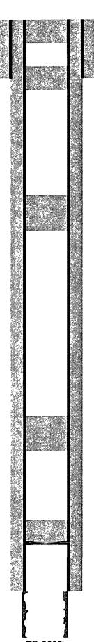
15" hole @ 312' 13-3/8" csg @ 312' w/ 175sx-TOC-Surf-Circ
