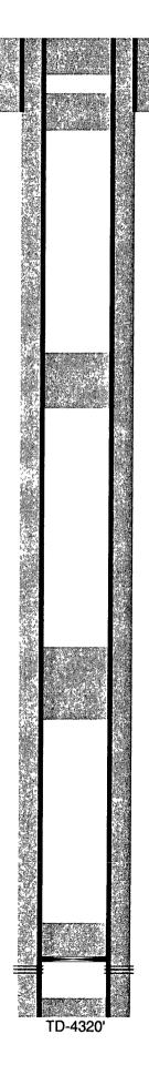
12-1/4" hole @ 363' 8-5/8" csg @ 363' w/ 350sx-TOC-Surf-Circ
