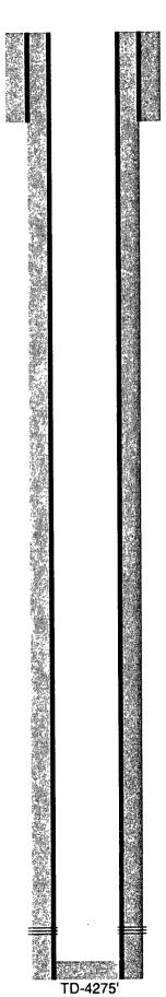
12-1/4" hole @ 394' 8-5/8" csg @ 394' w/ 300sx-TOC-Surf-Circ
