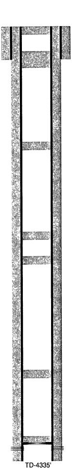
12-1/4" hole @ 335' 8-5/8" csg @ 335' w/ 250sx-TOC-Surf-Circ
