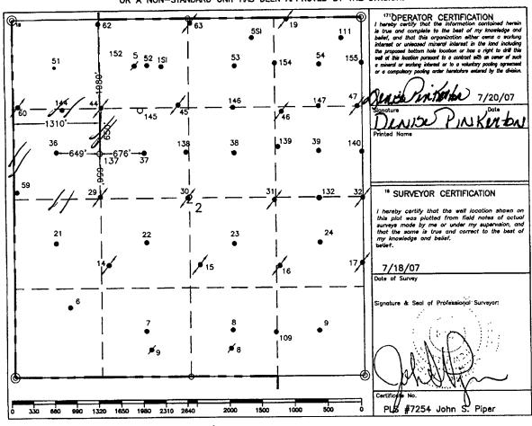
O = Staked Location • = Producing Well = Injection Well • = Water Supply Well • = Plugged & Abandon Well O = Found /4 Section Corner, 1" Iron Pipe & GLO B.C. ○ = Found Section Corner, 2 or 3" Iron Pipe & GLO B.C.
