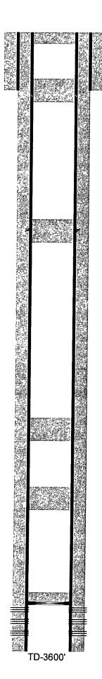
12-1/4" hole @ 314' 9-5/8" csg @ 314' w/ 300sx-TOC-Surf-Circ
