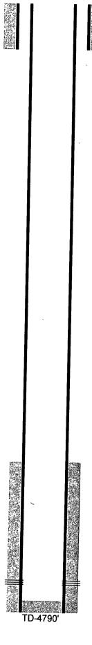
11" hole @ 390' 8-5/8" csg @ 390' w/ 300sx-TOC-Surf-Circ
