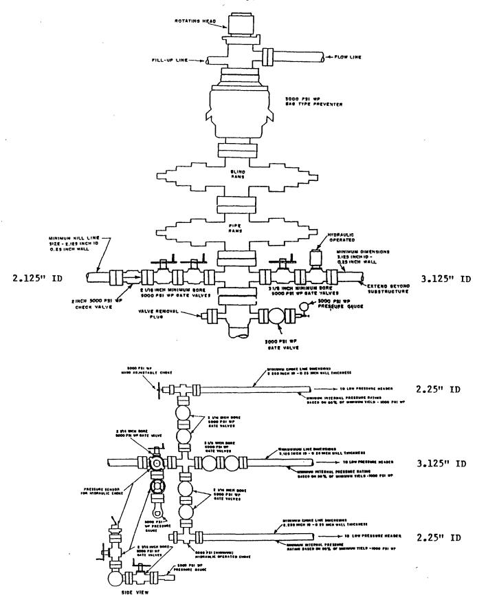
5000 PSI WORKING PRESSURE CHOKE MANIFOLD
