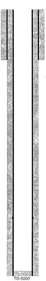
12-1/4" hole @ 840' 8-5/8" csg @ 840' w/ 500sx-TOC-Surf-Circ
