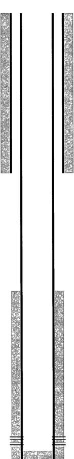
12-1/4" hole @ 1550' 8-5/8" csg @ 1550' w/ 400sx-TOC-Surf-Circ
