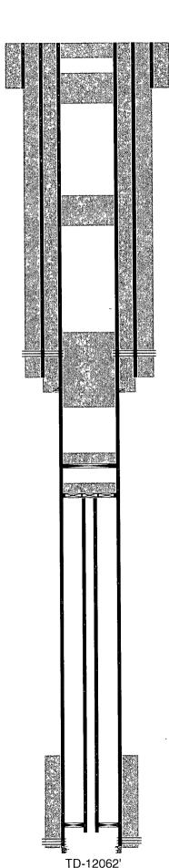
17" hole @ 460' 13-3/8" csg @ 460' w/ 475sx-TOC-Surf-Circ
