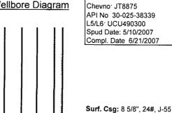
Set: @ 495' w/ 490 sks Hole Size: 12 1/4" Circ: Yes TOC: Surface TOC By: Circulated
