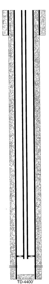
12-1/4" hole @ 380' 8-5/8" csg @ 380' w/ 250sx-TOC-Surf-Circ
