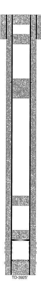
12-1/4" hole @ 398' 8-5/8" csg @ 398' w/ 260sx-TOC-Surf-Circ
