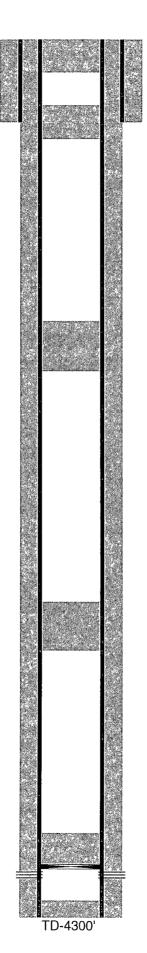
12-1/4" hole @ 388' 8-5/8" csg @ 388' w/ 350sx-TOC-Surf-Circ
