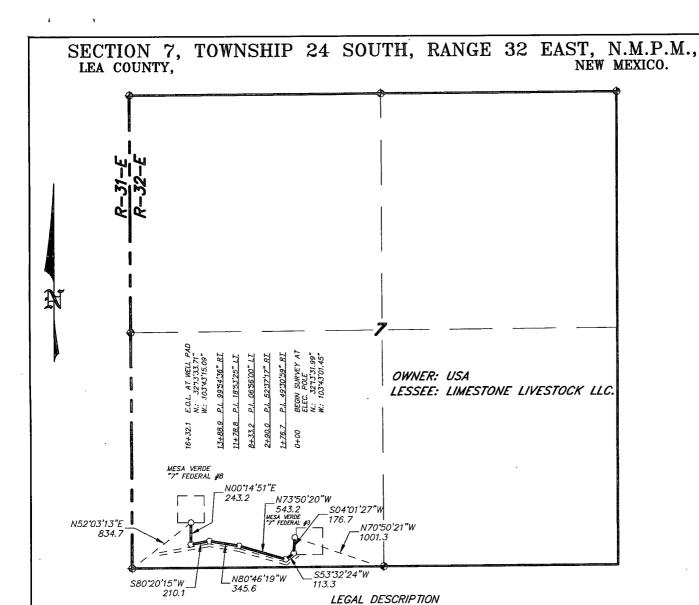
A STRIP OF LAND 30.0 FEET WIDE, LOCATED IN SECTION 7, TOWNSHIP 24 SOUTH, RANGE 32 EAST, N.M.P.M., LEA COUNTY, NEW MEXICO AND BEING 15.0 FEET LEFT AND RIGHT OF THE ABOVE PLATTED CENTERLINE SURVEY.
