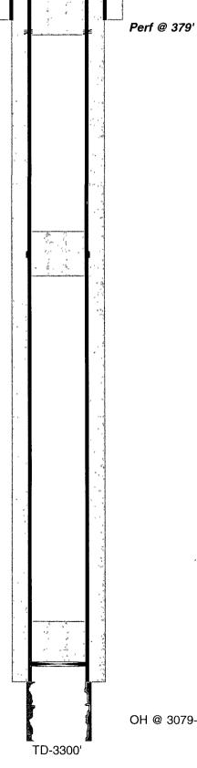
8-3/4" hole @ 3079' 7" csg @ 3079' DVT @ 1294' ~ 1st w/ 500sx-TOC-1290'-Calc 2nd w/ 250sx-TOC-400'-TS
