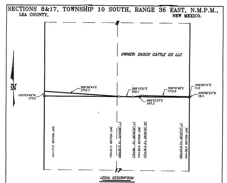
A STRIP OF LAND 30.0 FEET WIDE, LOCATED IN SECTIONS 8&17, TOWNSHIP 10 SOUTH, RANGE 36 EAST, N.M.P.M., LEA COUNTY, NEW MEXICO AND BEING 15.0 FEET LEFT AND RIGHT OF THE FOLLOWING DESCRIBED CENTERLINE SURVEY.
